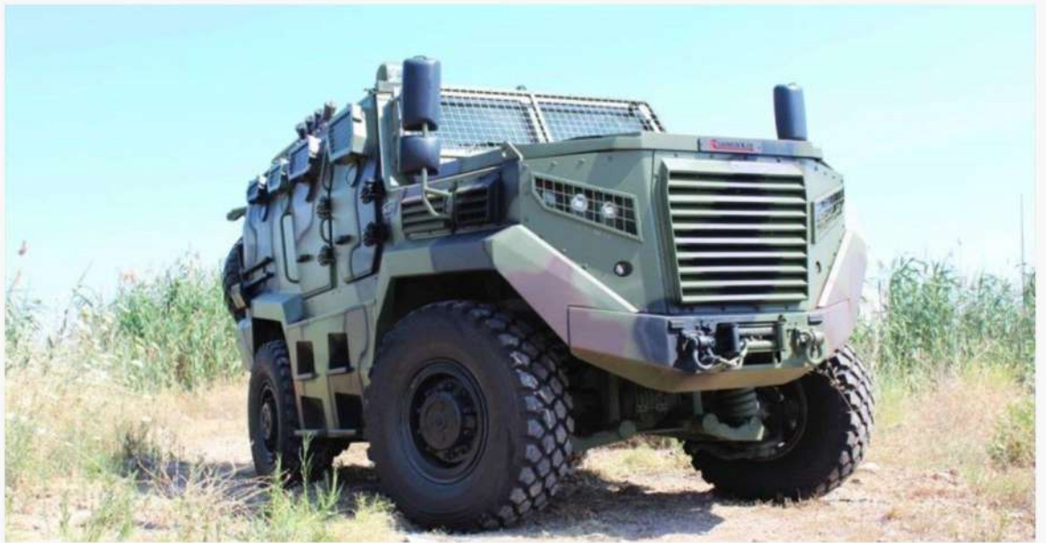
ARMoured PERSONAL CARRIER APC
