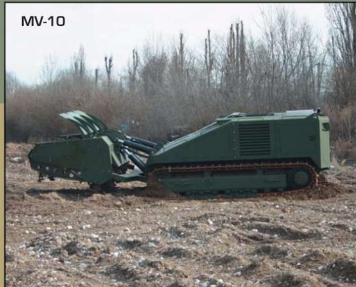
MV-10 flail tool attachment and tiller tool attachment
